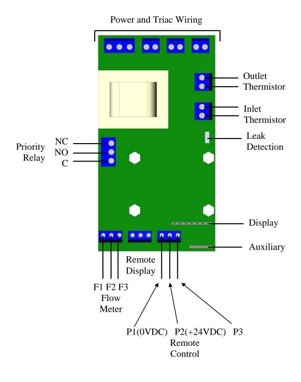
TK2000 Control Board Wiring Detail
