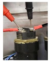
5. If all voltage readings are acceptable, proceed to <u>Check the Heating Elements</u>.
