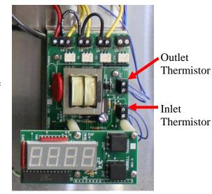
8. Repeat step 6 with the lower terminal block (inlet thermistor).
