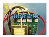
Proceed to test voltage on the other two terminal blocks **BLACK** cable to ground.
