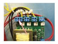
You will be getting a voltage reading at each of the **BLACK** cables to ensure there is current going to the electronic board as follows.
