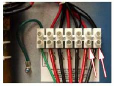
Using your multi meter probes with the setting at ACV (Alternating Current Volts) in the range of 250 + you need to place one probe on the lower screw of the BLACK cable of the terminal block, again from right to left and the other probe on the RED lower screw to the left of the BLACK cable. You should have a voltage reading somewhere in the 220+ range. Proceed to take the same readings on the next set of BLACK/RED screws. (the lower screws as before) Write down the Voltage below.
