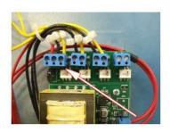
You will need to have your multi meter set to read Voltage (AC). We are going to measure the current going to each of the power supplies on the Electronic Board.
