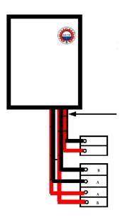
In this section you will check to ensure the cables supplied from the unit have been installed correctly into the service panel breakers supplied with the unit. If these cables are not connected correctly the unit will produce NO HOT WATER even though all the components are carrying voltage and the **RED** LED light turns on.
