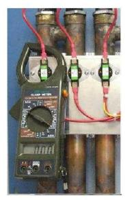
NOTE: Now perform this same test with the HOT WATER TURNED OFF. You should get a ZERO reading at each of the elements since the element should only draw amperage when there is a hot water tap opened. If you get an Amperage reading with the Hot Water TURNED OFF then the TRIAC(S) are bad and needs to be replaced.
